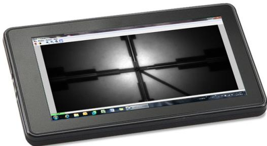
AlignCam mobile option comes with a Kindle Fire to allow the user to observe alignments while creating real-time adjustments.
