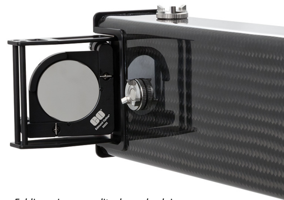
Folding mirror expedites beam buck-in process.
