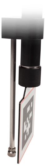
*Above*: A special "foot" on the vertical scale bar keeps the April tag off the ground, allowing the bar to lean against any vertical surface.
