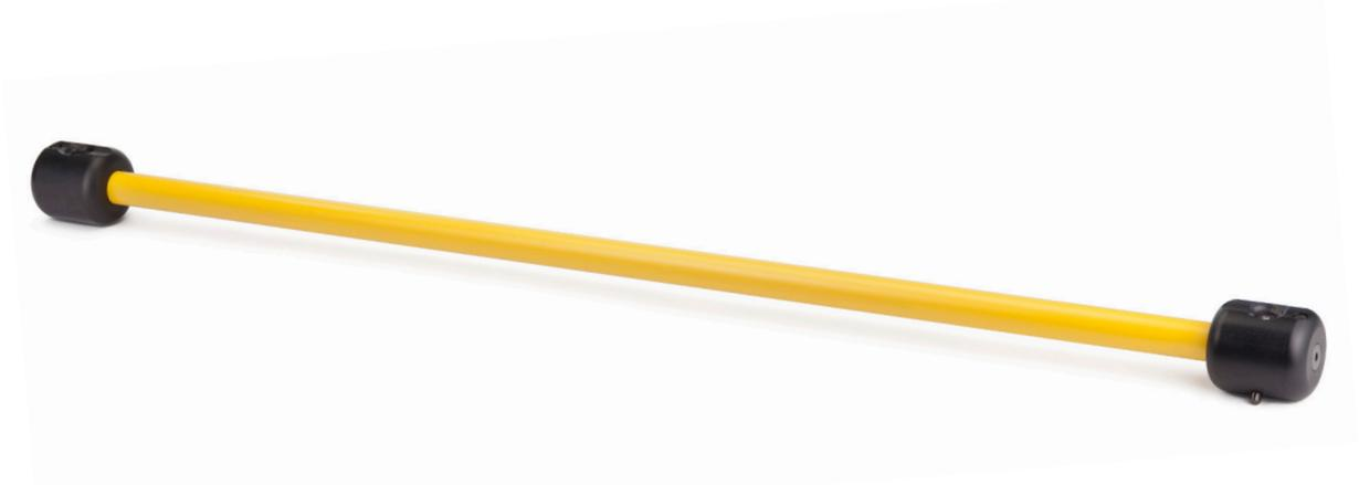
Integrated target holders on each end are positioned off-axis and allow the SMR to rotate 360° for easy visibility. A new 3-point mount constrains the bar in the field exactly as it is certified at the factory to assure the highest accuracy possible.
