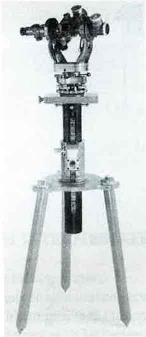
Model 810 shown with collar in upright position on tribrach, long legs (26"), and long intermediate tube (21"). Instrument is a Brunson model 376-RHN.
